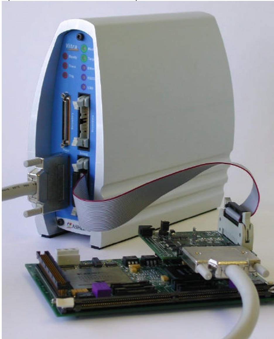
The Ashling Universal VITRA Emulator with full NEXUS Class 3 support.
