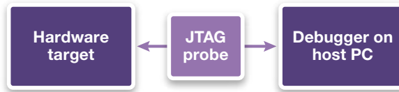
Figure 2: An example of using JTAG to debug an embedded target
