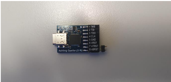
Figure 9. The Opella-LD Blanking Pins (pins 7 and 8)
