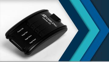
**Opella-XD** is Ashling's high-performance Debug Probe for embedded development with support for multiple target architectures including RISC-V, Arm, MIPS (P8700 & 18500) & Synopsys ARC & ARC-V powered systems.
