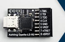
**Opella-LD** is Ashling's low-cost Debug Probe for embedded development with support for multiple target architectures including RISC-V & Arm powered systems.
